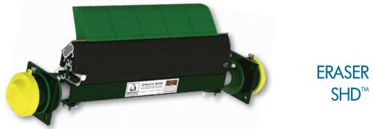
The Eraser SHD utilizes the Super Eraser mainframe and Safe Torque tensioners paired with an 11.25" tall replaceable tip blade. A mine duty design, this heavy-duty system allows for only the 6" blade tip sections to be replaced when they become worn, rather than the entire blade length.
