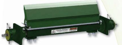
The Micro Eraser is your answer for portable equipment with tight clearance issues. Designed with our 6" tall polyurethane blade, it works best on belts up to 48" wide with head pulleys of 28" diameter or less. This economical but powerful system uses our patented Perma-Torque™ tensioner.
